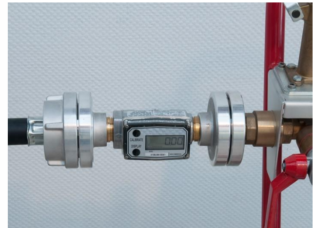
Flowmeter for small volume flows
